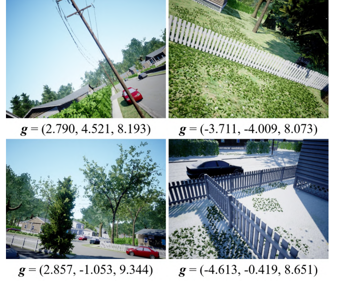
Fig. 2: Examples of datasets. The dataset consists of images and correspond gravity vectors \mathbf{g} [m/s 2 ] in the camera frame. These data are collected in “Neighborhood” of AirSim. The camera pose and weather parameters are randomized for creating a dataset. Road in the lower right image is covered by snow.
