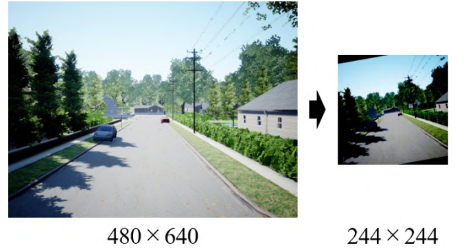
Fig. 3: Example of a transformed image. An image is randomly rotated according to \alpha . This example shows an image when \alpha = 10 deg. It is also resized, and is normalized.
