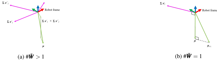
Fig. 9 Gravity vector estimation. When the number of the clusters is more than one, the gravity vector \boldsymbol{\mu} is estimated as (a). When the number of the clusters is only one, the gravity vector \boldsymbol{\mu} is estimated as (b).
